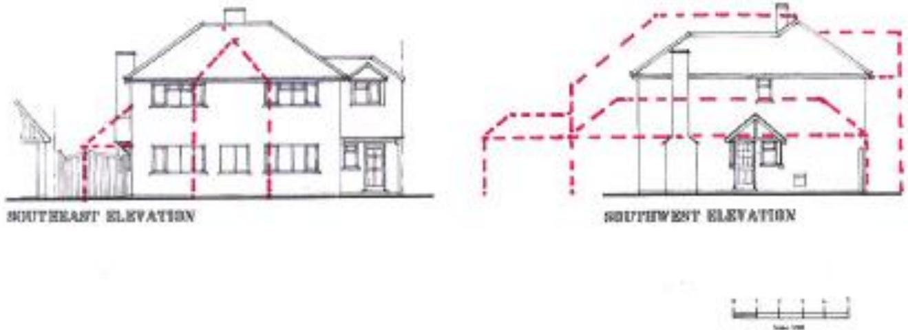
Proposed scheme overlaid on existing SE and SW elevations
