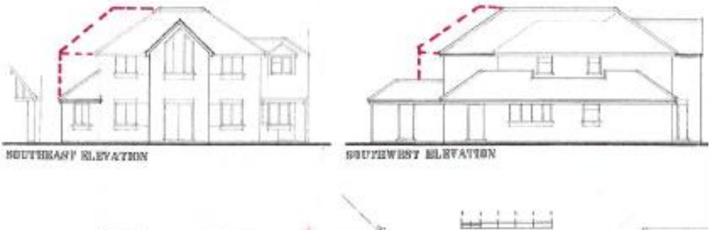
Refused scheme overlaid on proposed SE and SW elevations
